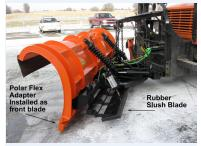
Clear Roads funded the development of <u>innovative prototype</u> <u>snowplows</u> capable of tackling a range of winter road conditions using multiple plow blades.
