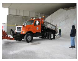
The Clear Roads <u>calibration guide</u> advises operators to raise the truck bed to an operational elevation for calibration.
