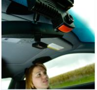
The DriveCam event-triggered video recording system was mounted on the windshield behind the rearview mirror of each participant's vehicle.
