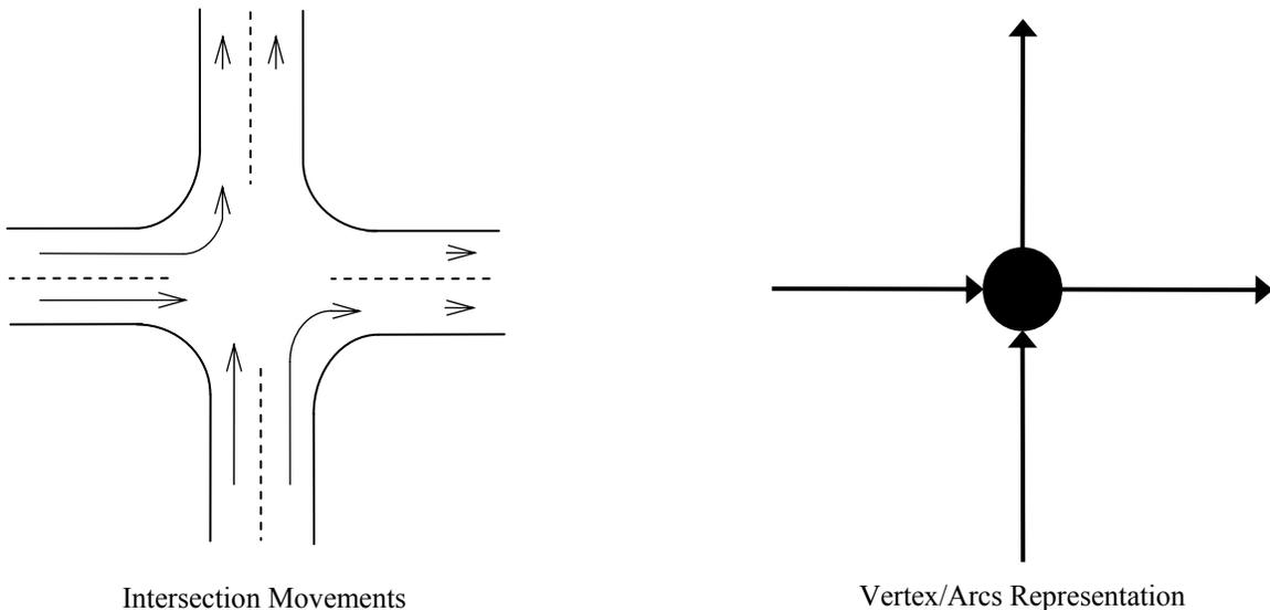
Figure 5.1 Graph Theoretic Representation of an Intersection
