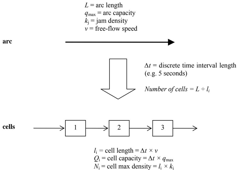
Figure 4.5 Transforming Arcs into Cells
