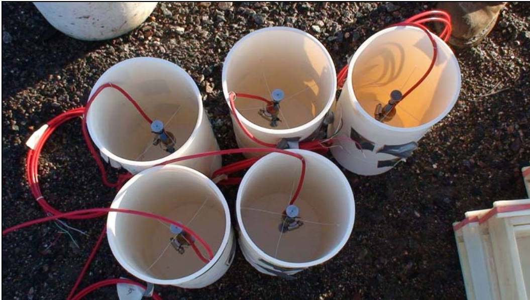
Figure 2. Orientation of strain gauges in CTE cylinders.
