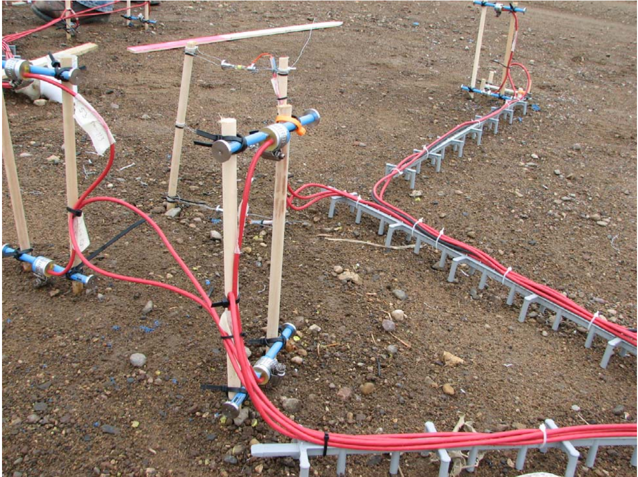
Figure E5. Vibrating wire strain gauges.
