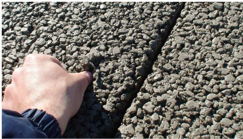
Figure 41. Cell 85 Pervious Concrete Still Soft after 24 Hours
