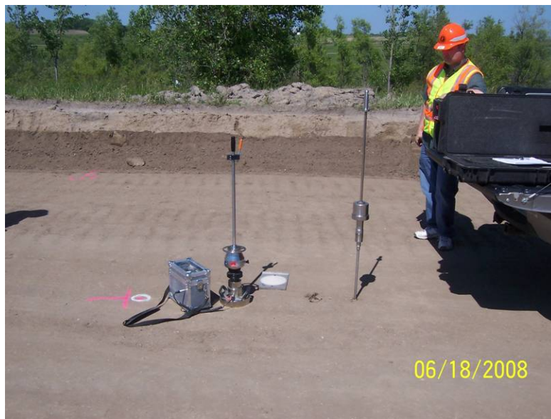
Figure 30. LWD and DCP Field Testing
