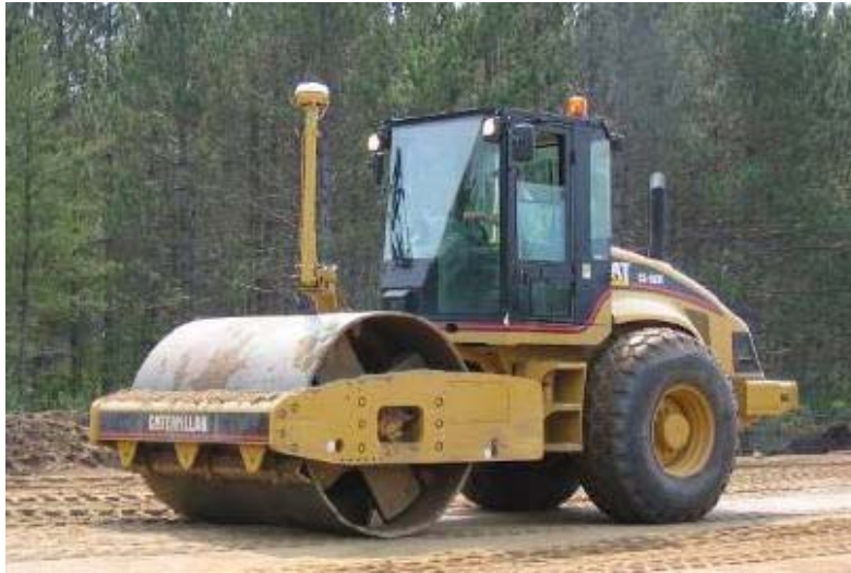
Figure 31. Caterpillar CS-563 Intelligent Compaction Roller
