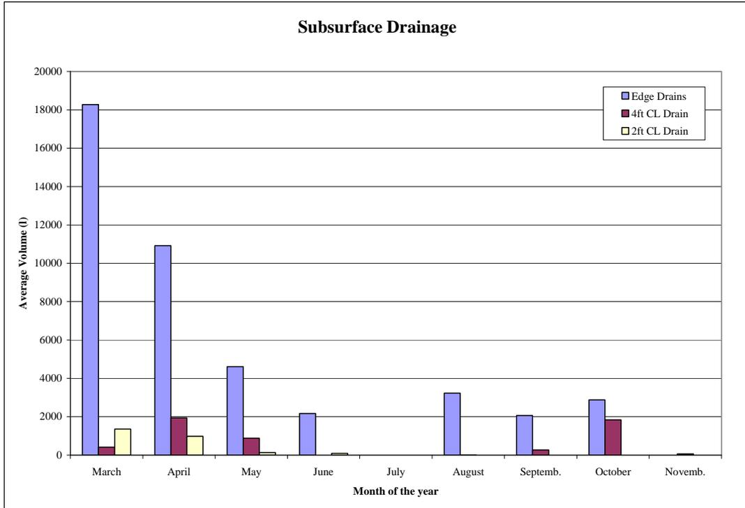
**Figure 3.2 Average drained volumes from edge/centerline drains (l) – 2007**
