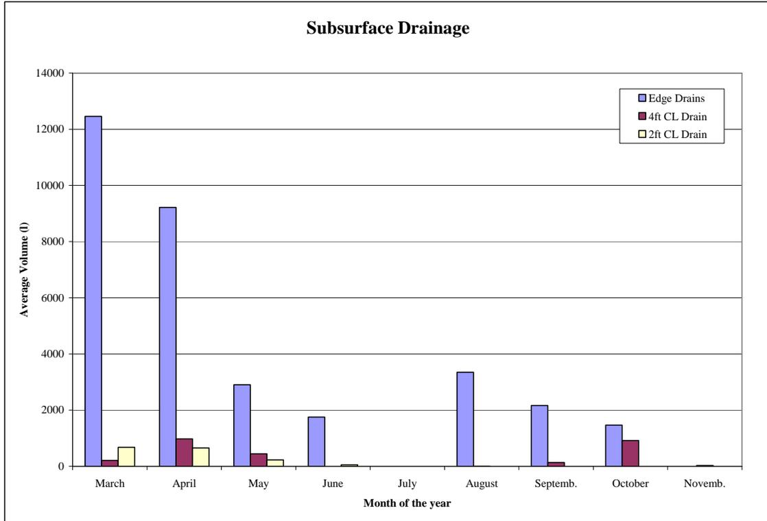
**Figure 3.3 Average drained volumes from edge/centerline drains (l) – 2006/2007**
