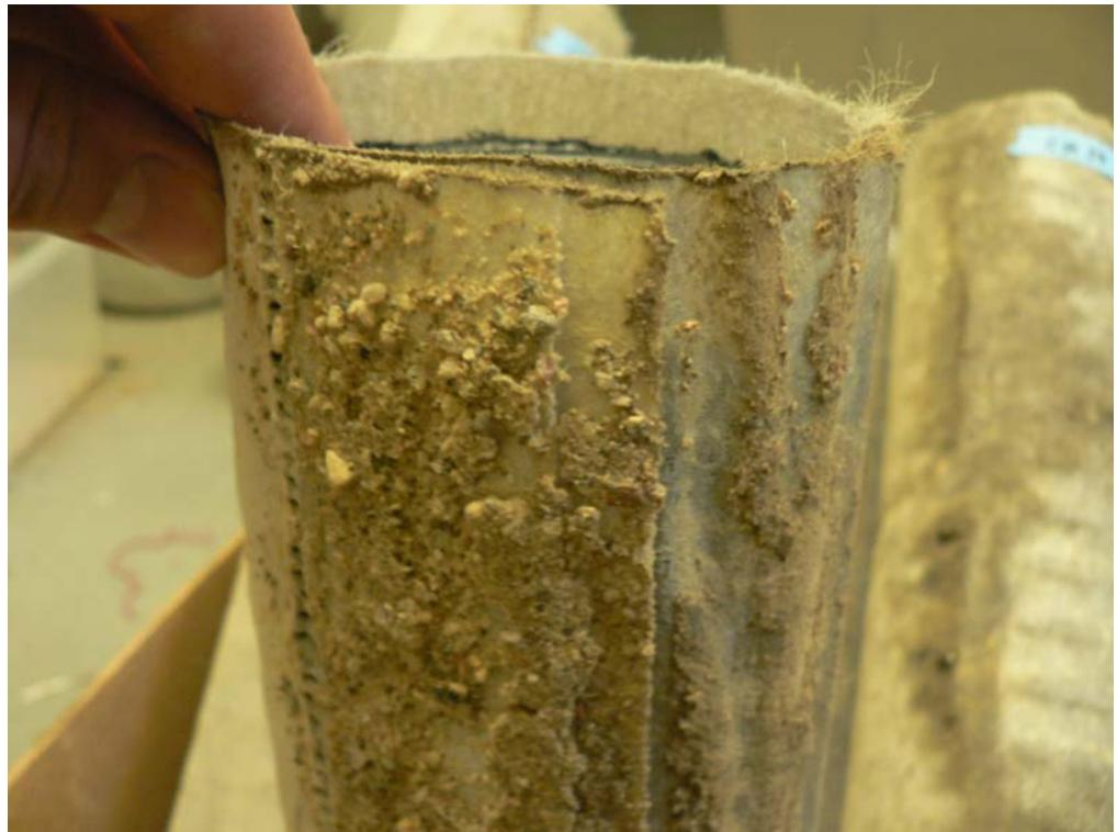
**Figure 7.9** The geofabric of the edgerain at site B on CR 32
