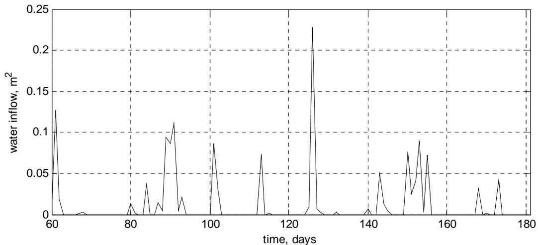
**Figure 6.4 Rate of water infiltrating into the roadway shoulder ( $m^3$  water /m roadway)**
