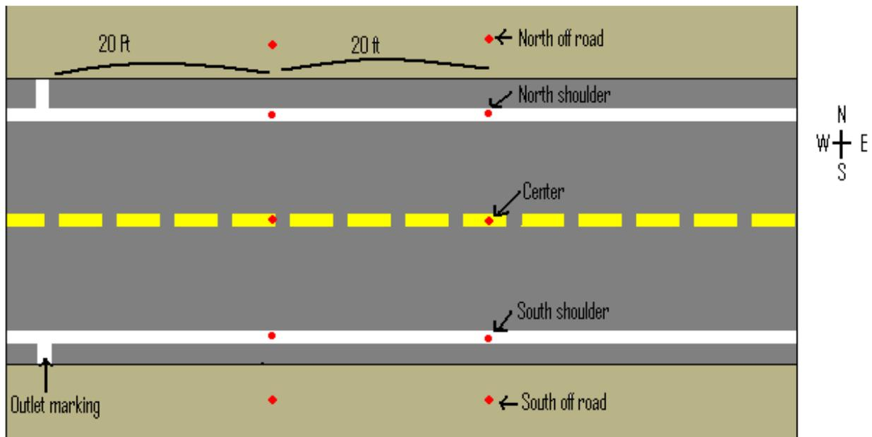
**Figure 4.1 Measurement scheme for the EM38 induction instrument**
