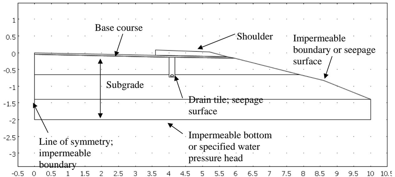
**Figure 6.1 Typical cross-sectional view of edgedrain geometry**
