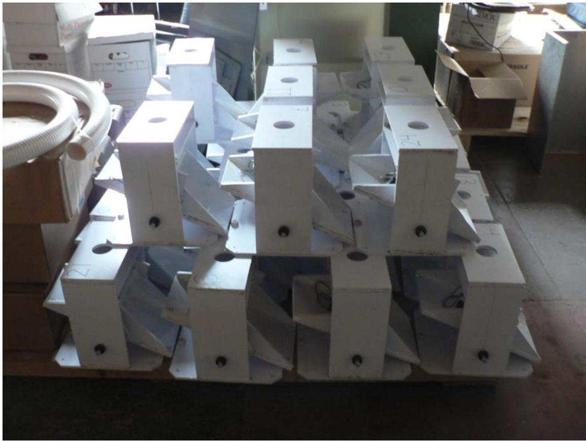
**Figure A.1 The inventory of tipping buckets constructed for the project**
