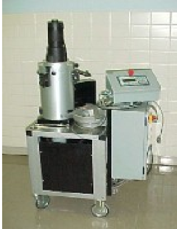
Figure 4.5 Superpave gyratory compactor used
