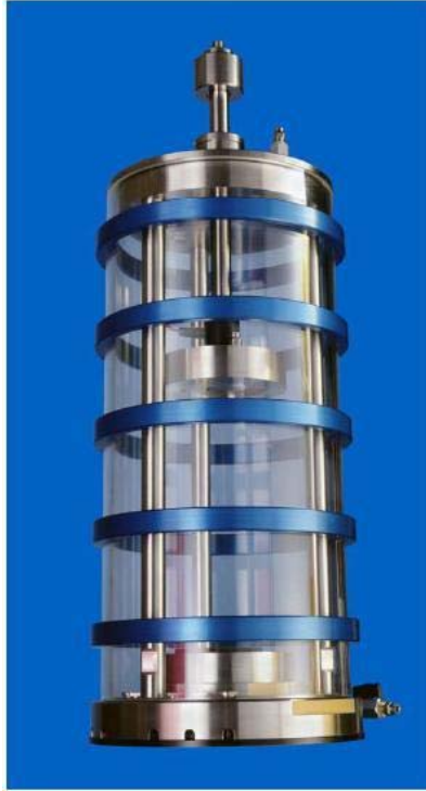
Figure B.1 Triaxial pressure chamber at NDSU.
