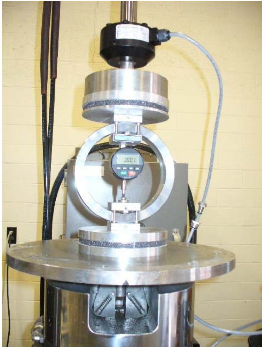
Figure B.5 Load cell calibration setup
