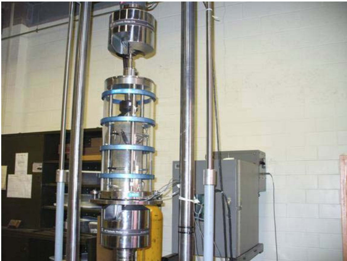
Figure 4.7 Resilient modulus sample during testing on the MTS
