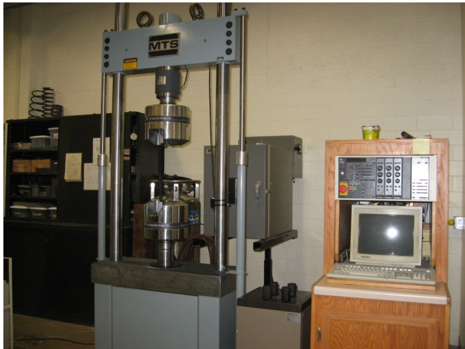
Figure B.2 MTS electro-hydraulic loading frame at NDSU.
