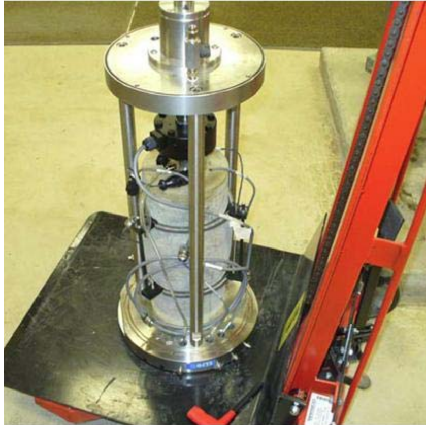
Figure 4.8 Resilient modulus sample with the internal load cell and LVDTs connected around the sample
