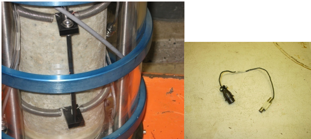
Figure B.4 LVDT (on the right) and LVDT holder (on the left) at NDSU.
