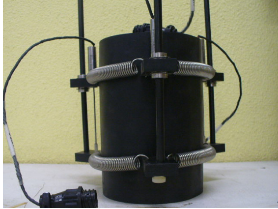
Figure B.7 Synthetic rubber specimen and LVDTs
