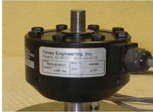
Figure B.3 5000 Lb electronic load cell at NDSU.
