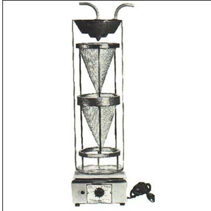
Figure 4.4 Asphalt extraction apparatus
