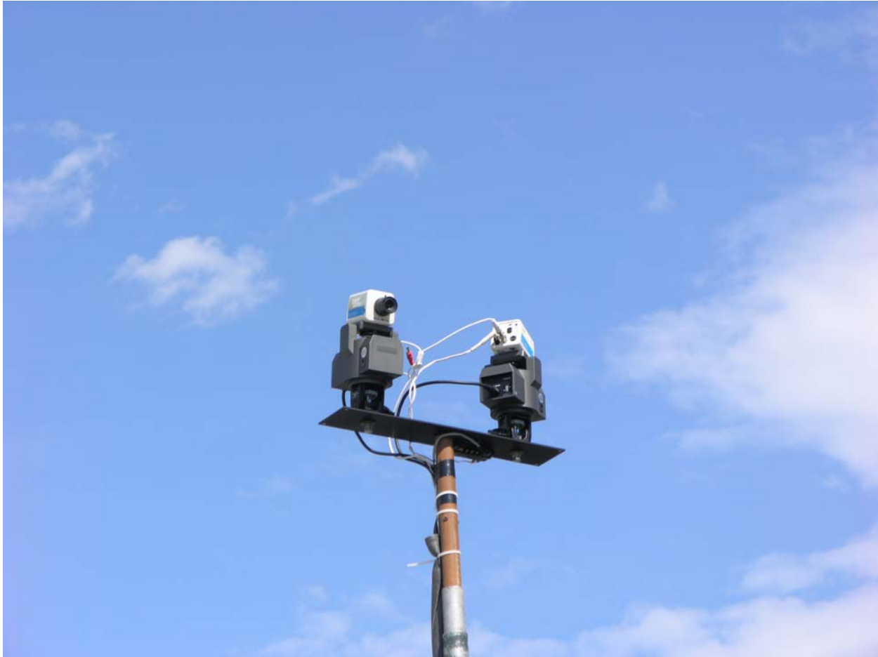
Figure 3. Close-up of cameras affixed to pan-and-tilt mounts at apex of boom.
