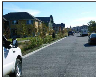
Porous Concrete – low volume residential street
