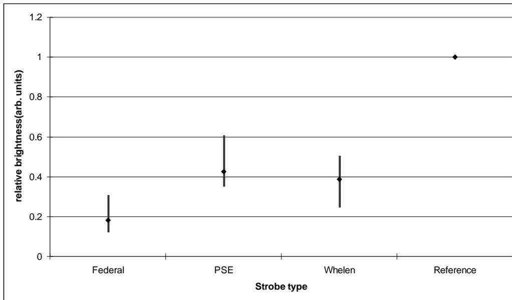
**Figure 3. 11. Perceived brightness comparison – MDB method**
