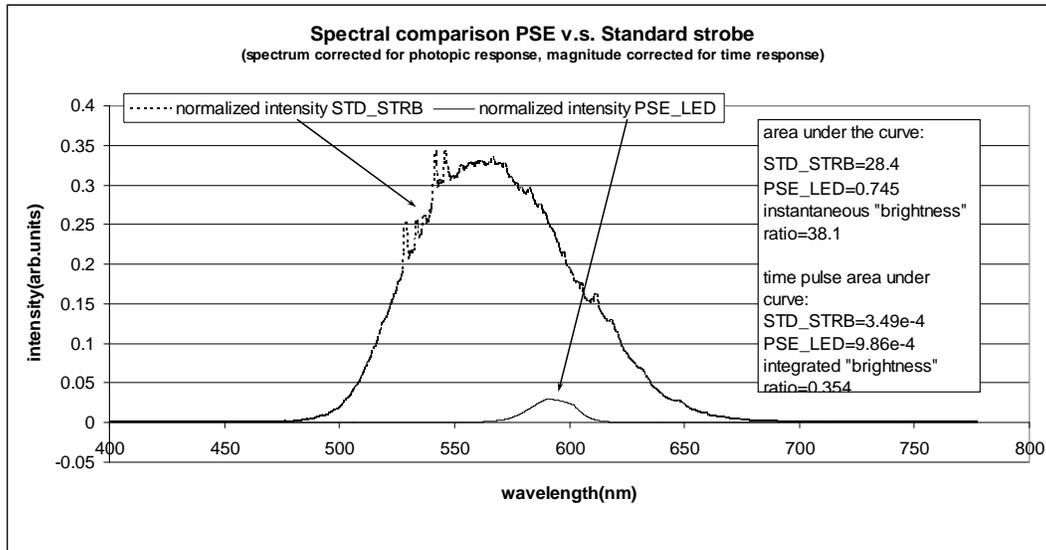
**Figure 3. 12. Color spectrum – LED v.s. standard strobe**
