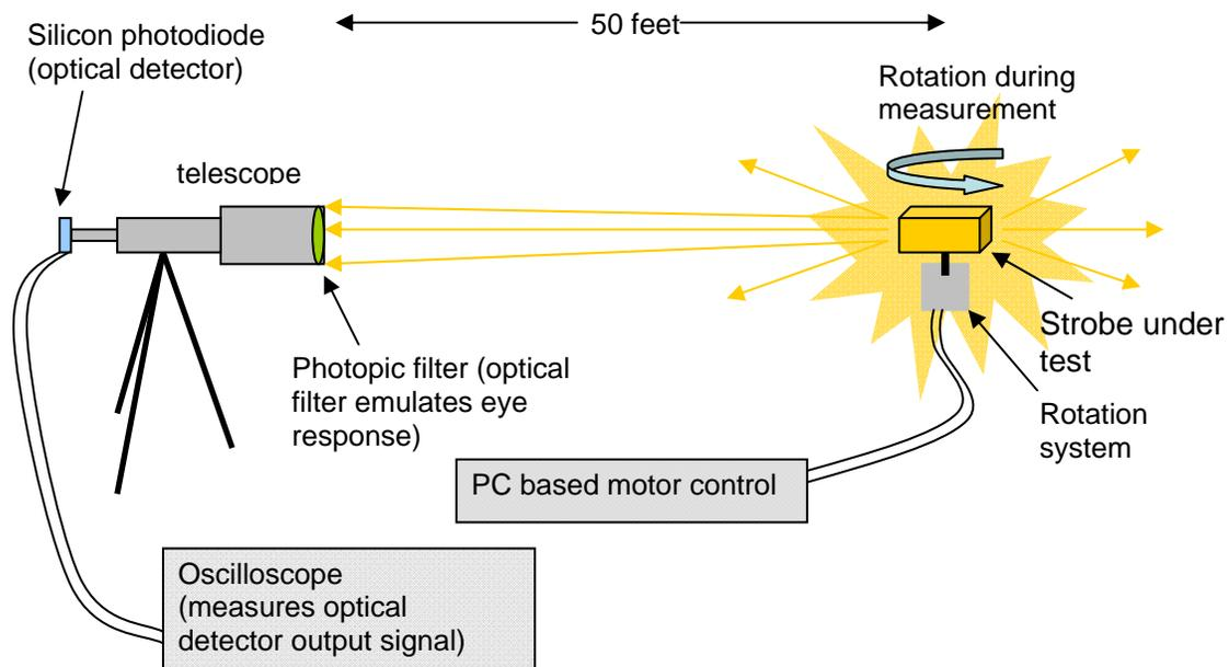
**Figure 2. 1. Optical power measurement system sketch**
