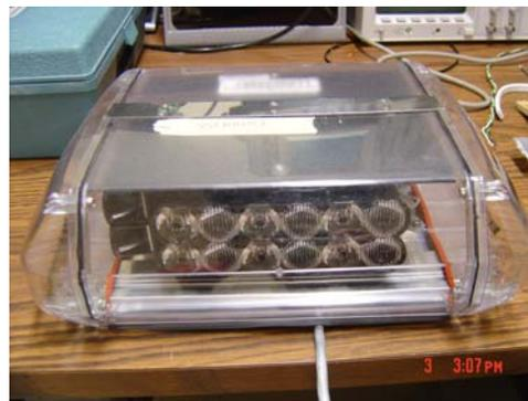
**Figure 1. 6. Photo of one of the LED strobes from PSE used in this study**
