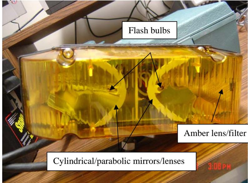
**Figure 1. 3. HID Standard strobe tested in this study**
