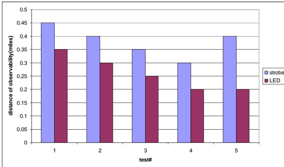
**Figure 3. 10. Distance of observability data for ice/snow coated standard and Whelen LED strobes**
