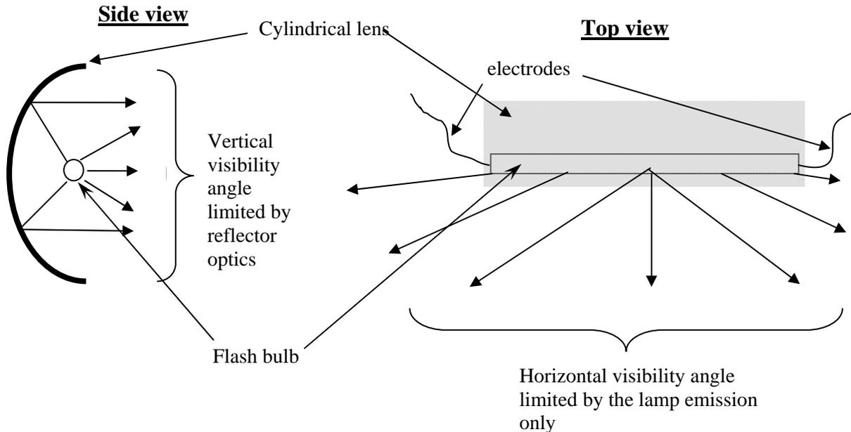
**Figure 1. 4. Sketch highlighting the physical and optical structure of a single light assembly for the standard strobe**
