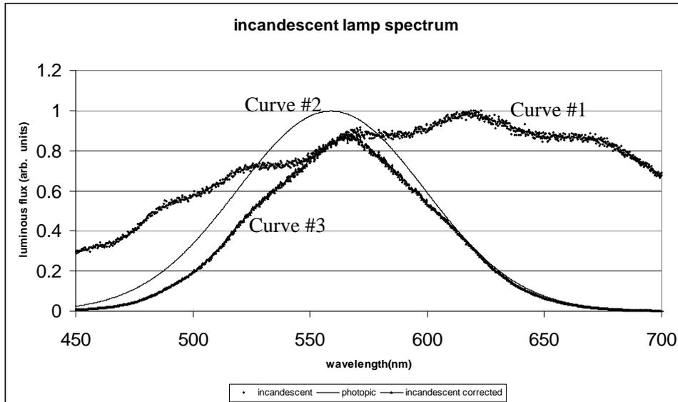
**Figure 1. 1. Incandescent lamp spectral characteristics and eye response**
