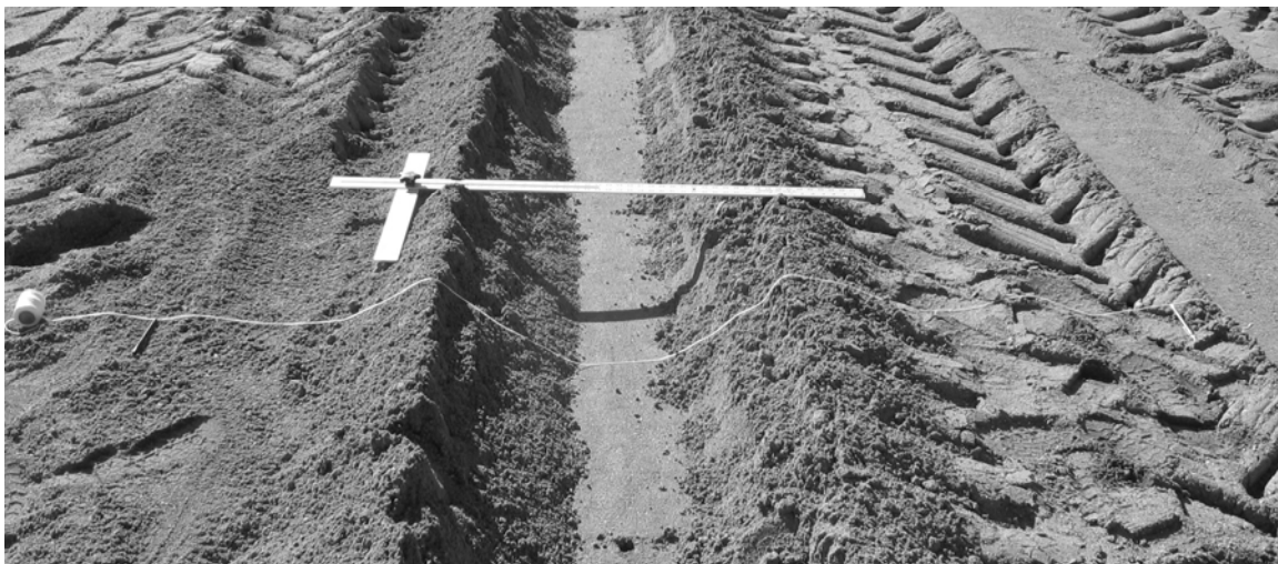
Figure 5.12. Large rut at site with granular soil
