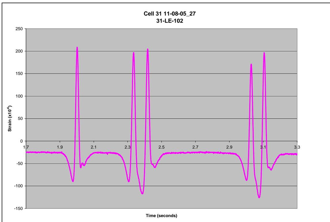
**Figure 1.1** Typical signal response from strain sensor during pavement load testing.
