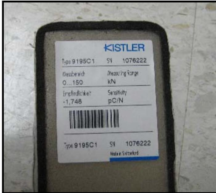
**Figure 62:** 9195 sensors with sensitivity measure
