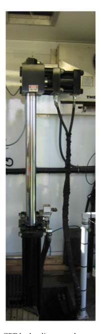
Figure 3.2. CPT hydraulic cone advancement system.
