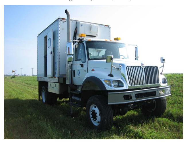
Figure 3.1. Cone penetration test (CPT) truck.
