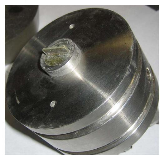
Figure 2.1. Bender elements housed in resilient modulus platens.
