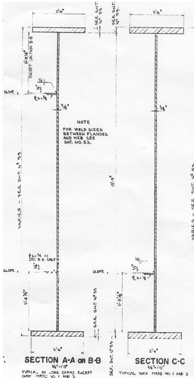
Figure 8.4 Transverse stiffener web gap – girders (Bridge # 9330)
