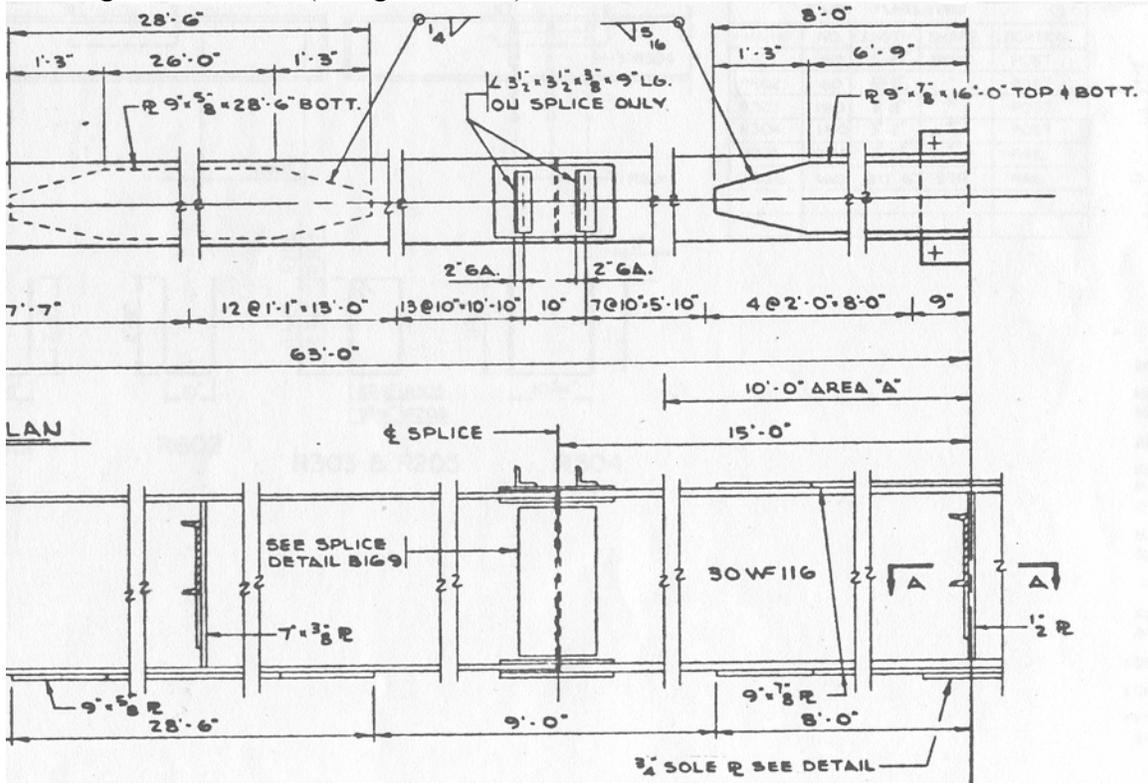
Figure 8.7 Partial length cover plate (Bridge # 02803)
