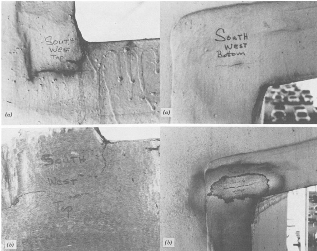
**Figure 2.21** Lamellar cracks in girder tension flanges (left) and compression flanges (right) (Fisher 1984)
