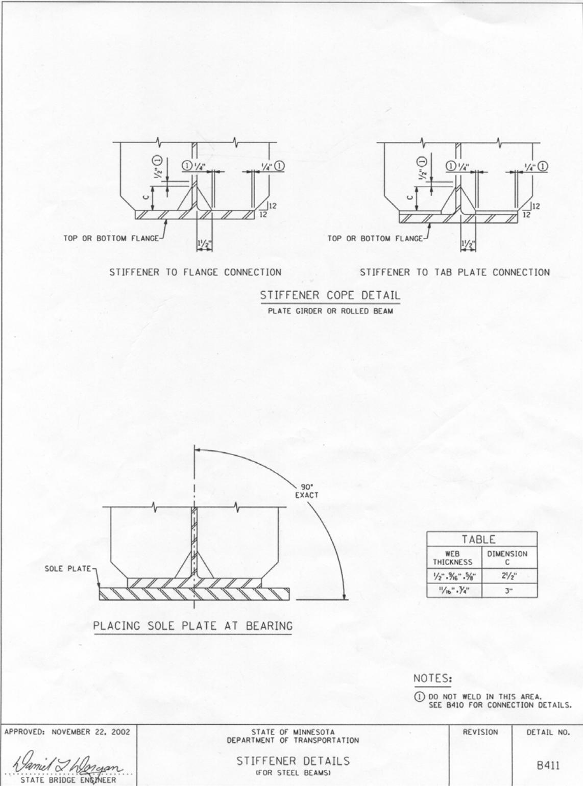
Figure 4.3 Standard weld termination distances for stiffeners (Mn/DOT, 2002)
