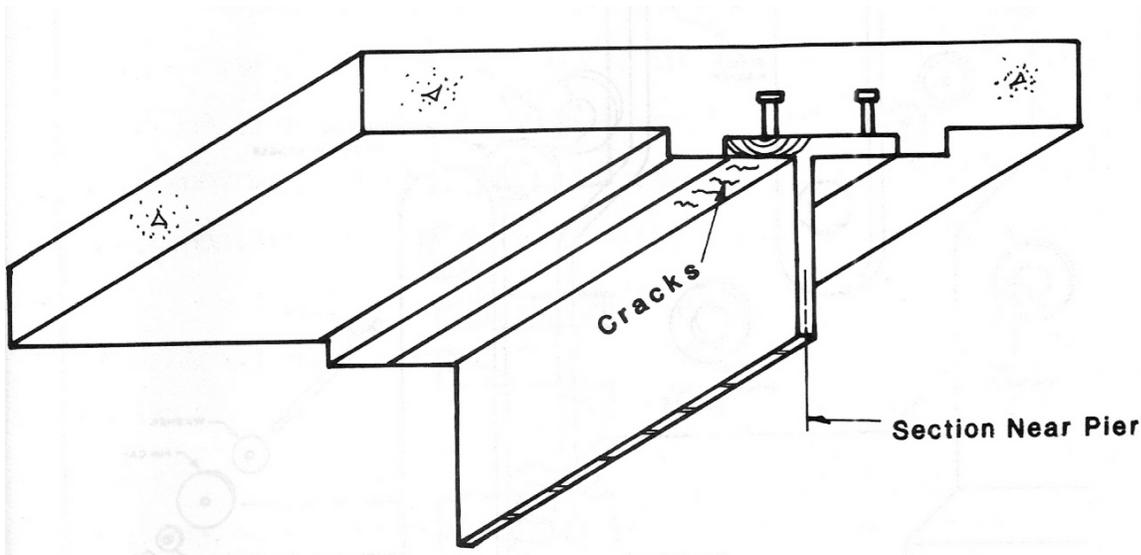
**Figure 3.1** Composite section cracks from studs (FHWA 1986)
