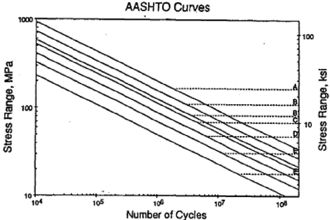
Figure 2.1 AASHTO S-N curves for detail classification A through E'
