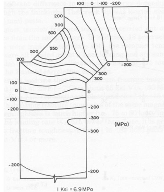
**Figure 2.19** Stress concentration diagram for corner weld from residual heating stresses (Fisher 1984)
