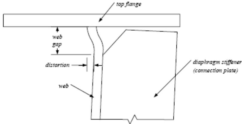
**Figure 2.5** Relationship between variables for differential deflection and web gap distortion (Li, 2005)
