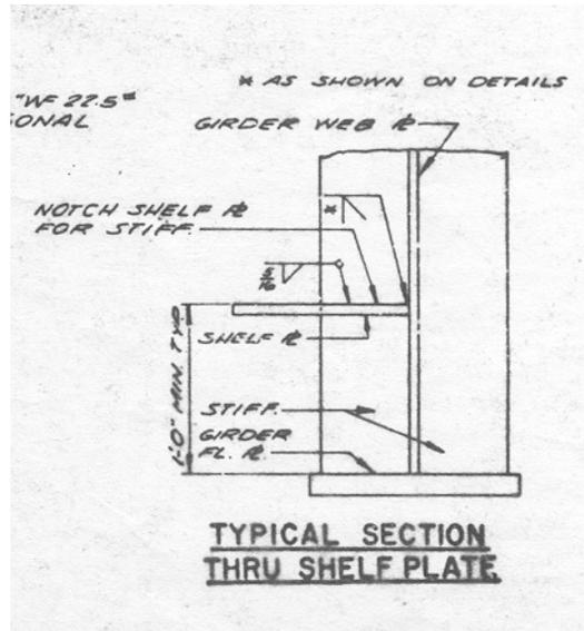
Figure 8.10 Shelf plate welded to girder web – welding detail (Bridge # 9320)
