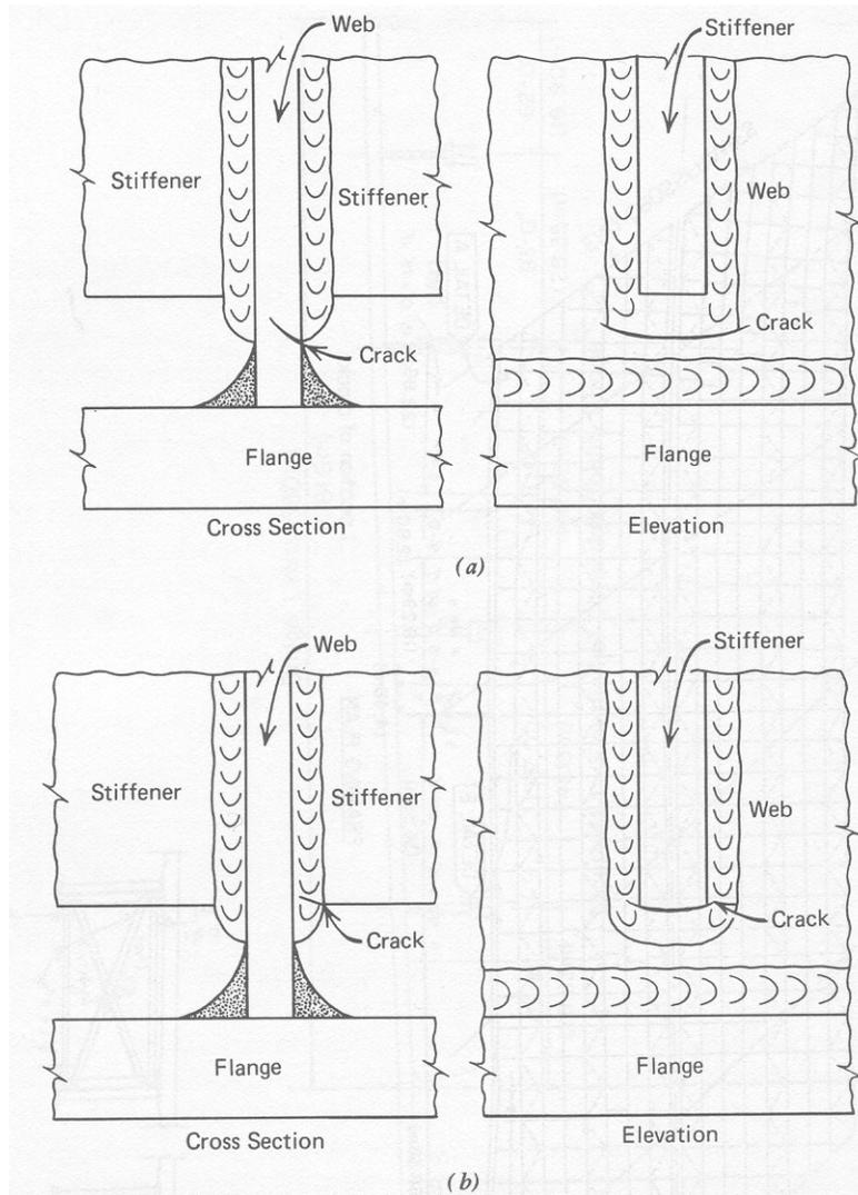
**Figure 2.6** Transverse stiffener web gap cracks on the I-90 Bridge (Fisher 1984)
