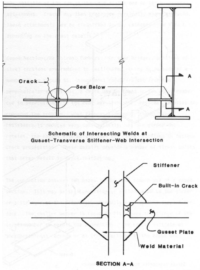
**Figure 2.2** Intersecting stiffeners weld detail (Fisher 1981)
