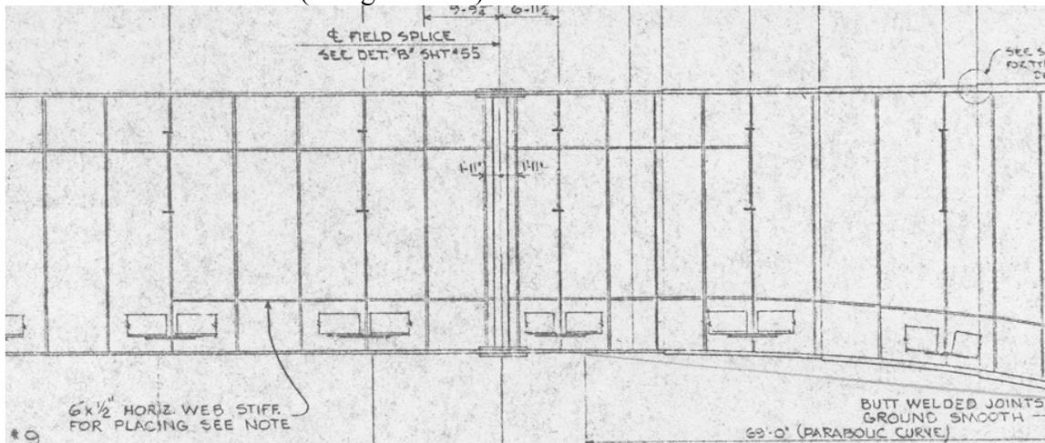
Figure 8.12 Welded horizontal stiffener (Bridge #9800)
