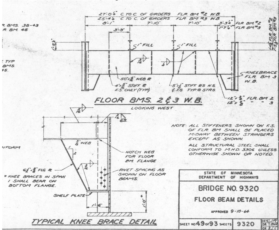
Figure 8.8 Shelf plate welded to girder web (Bridge # 9320)
