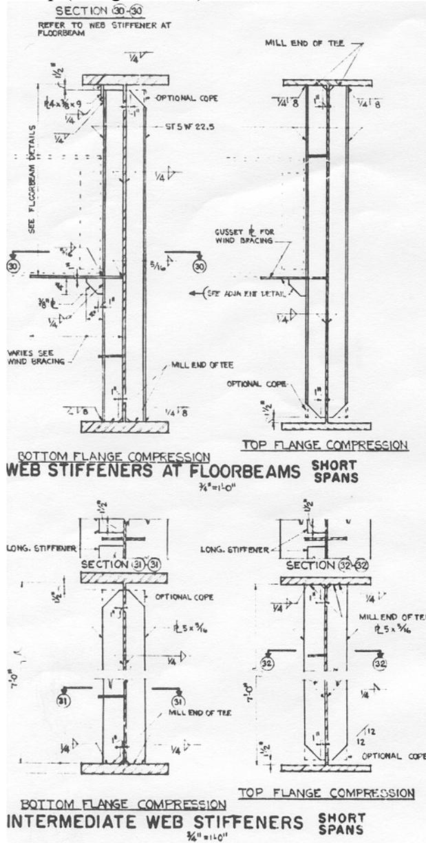
Figure 8.3 Transverse stiffener web gap (Bridge # 9330)
