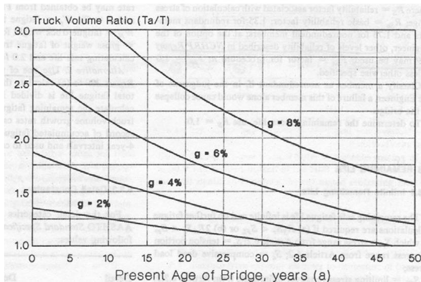
**Figure 2.23** Growth rate graphs for determination of  $T_a$  value (Moses et al., 1987)
