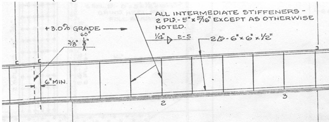
Figure 8.20 Intermittent weld (Bridge # 6566)
