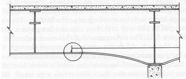
**Figure 2.13** Cracked end of haunch insert on Aquasabon River Bridge (Fisher 1984)
