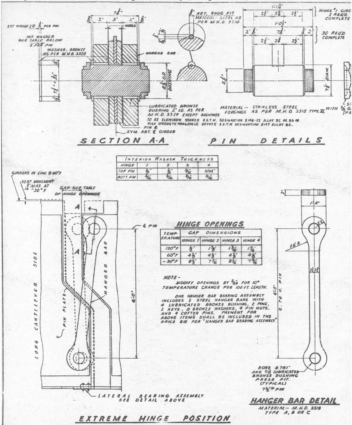
Figure 8.17 Pin and eyebars truss or pin and hanger assembly (Bridge # 9320)
