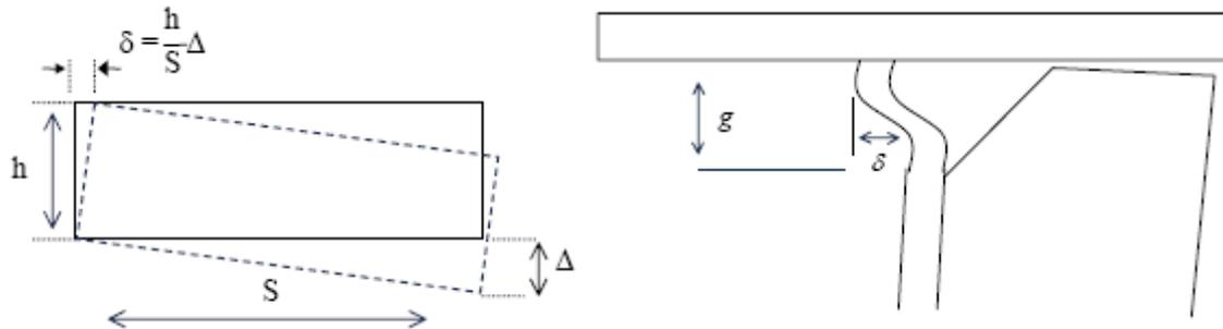
Figure 2.24 Distortional fatigue geometry (Jajich, 2000)
