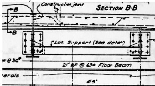
Figure 8.11 Floor-beam bracket (Bridge # 5947)
