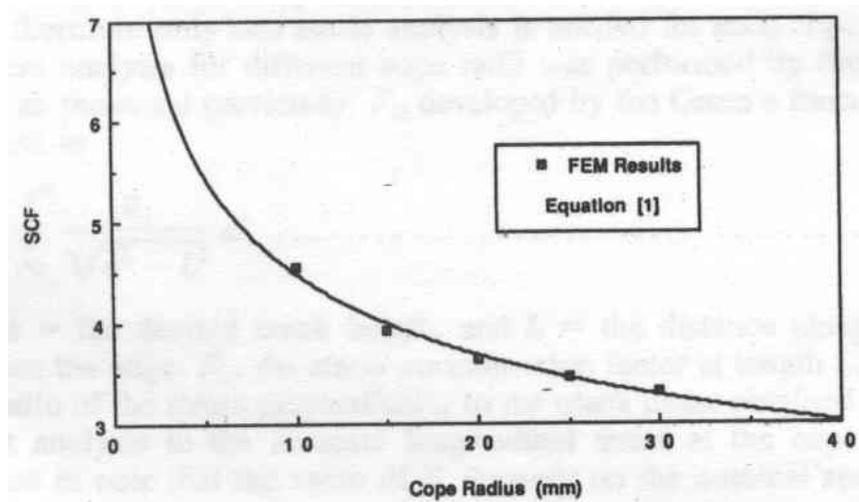
**Figure 4.2** Stress concentration factors for various cope radii (Yam, 1990)
