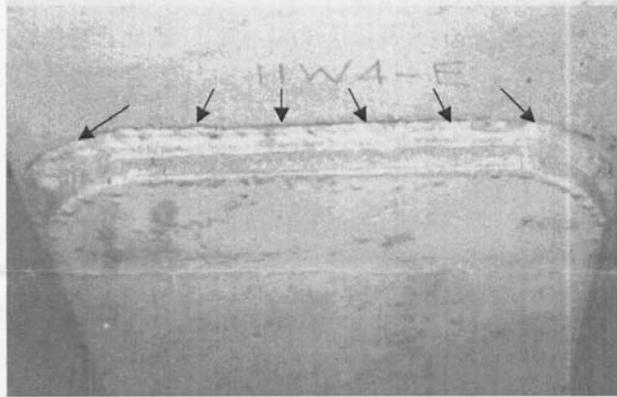
2 *Stringer to floor beam (truss) brackets* – Cracking occurs in the angles connecting floor beams to other elements. Cracks can occur anywhere within the angle connector.
