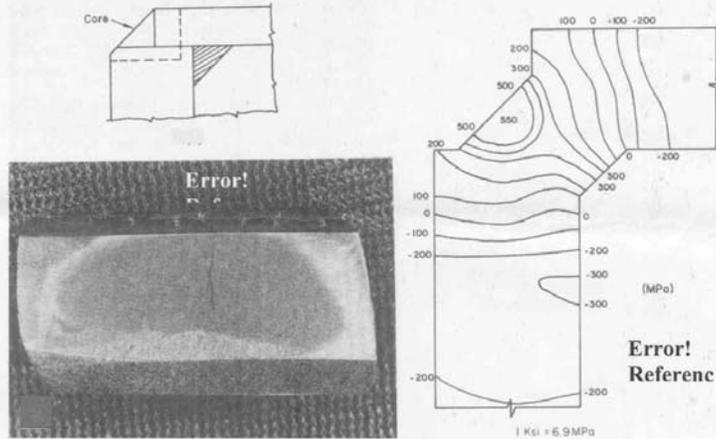
0 Lamellar Tearing – Separation of layers of metal *within* a solid piece. Cracking is usually found in highly restrained members or in cantilevers.
