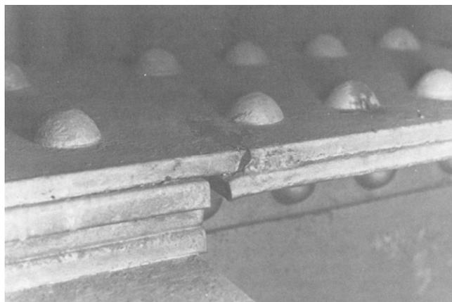
**Figure 2.16** Crack originating at tack weld through tie plate of Lehigh River Bridge (Fisher 1984)
