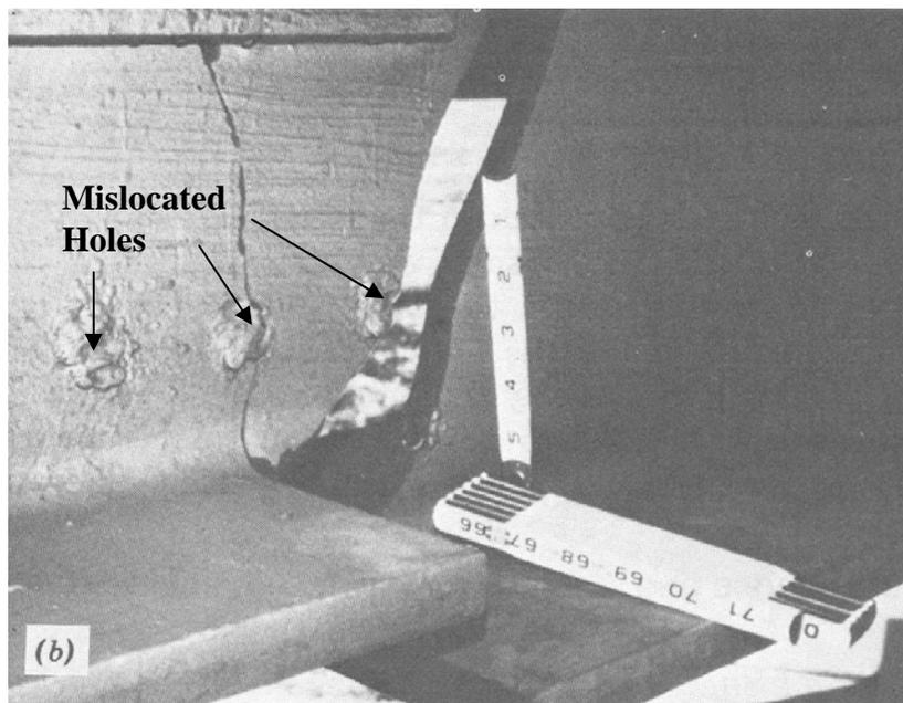
**Figure 3.2** Cracking at mislocated bolt holes of Highway 28 Bridge over I-57 (Fisher 1984)
