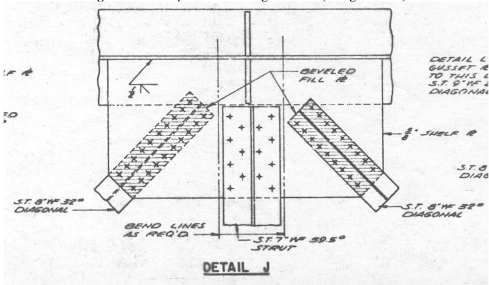
Figure 8.9 Shelf plate welded to girder web – plan view (Bridge # 9320)
