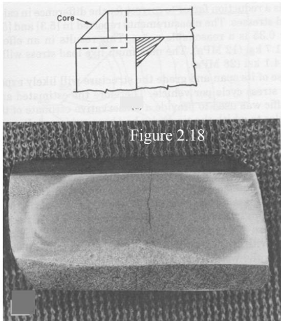
**Figure 2.18** Core of cracked section of corner weld from Gulf Outlet Bridge box girder (Fisher 1984)
