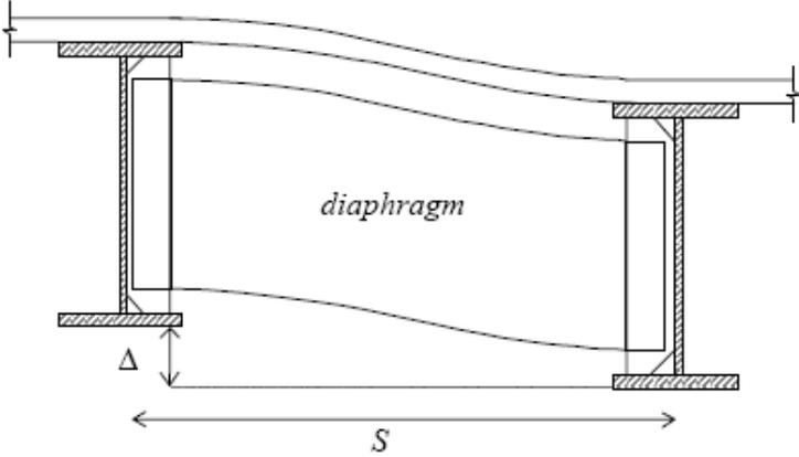
**Figure 2.4** Differential girder displacement resulting in web rotations (Li, 2005)
