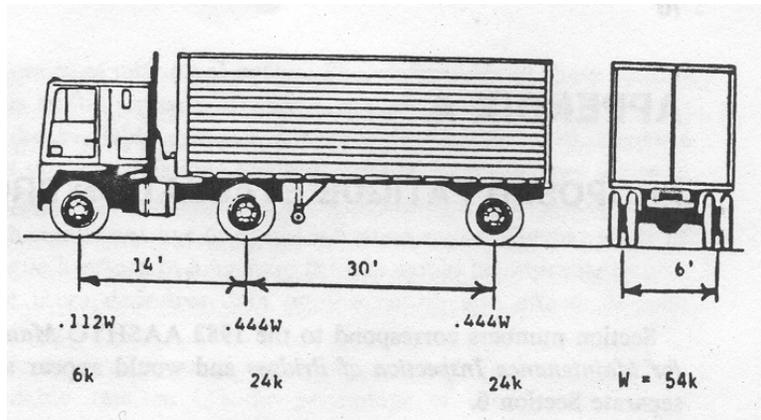
**Figure 2.22** Standard fatigue truck geometry and loading (Moses et al., 1987)
