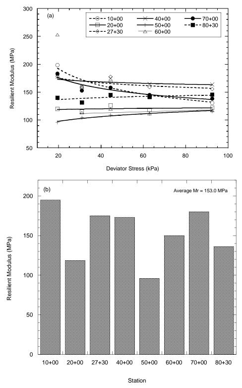
Fig. 21 Resilient modulus of mixture of fly-ash and gravelly soil prepared in the field.
