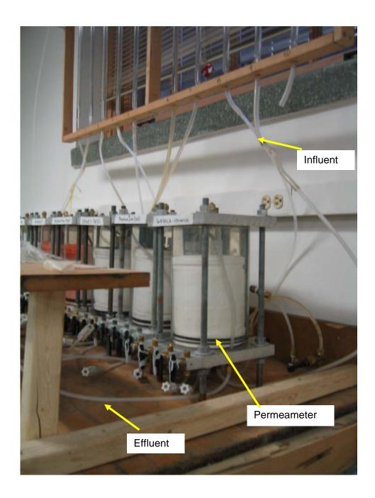
Fig. 6 Column leach test experimental setup
