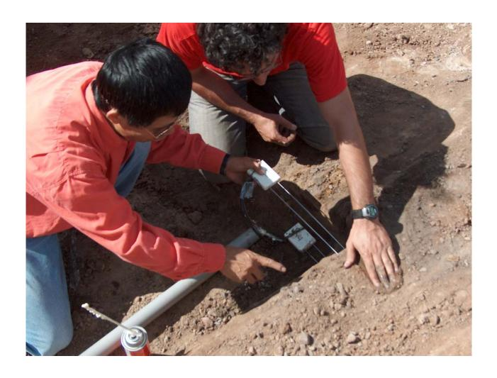
Fig A18. Installation of volumetric water content and temperature sensors into subgrade and RSG in lysimeter pit Sensor 1 is in subgrade and Sensor 2 is in RSG.
