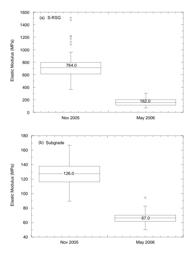
Fig. 27 Statistical evaluation of Elastic moduli back-calculated from FWD tests by using MODULUS 6.0 software. (a) S-RSG (b) Subgrade.
