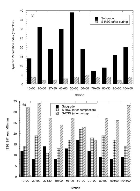
Fig. 23 (a) Dynamic penetration index (DPI) of subgrade and S-RSG soil prepared in the field after 7 d of curing, (b) Soil stiffness gauge stiffness of subgrade, S-RSG after compaction and after 7 of curing
