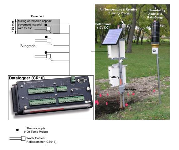
Fig. B4. Layout of field instrumentation.
