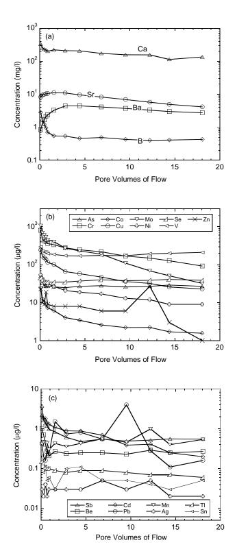
Fig. 19 Concentrations of trace elements in effluent from CLT on CH5 (Chisago Station 5): elements with peak concentrations (a) exceeding 1 mg/L, (b) exceeding 10  $\mu$ g/L, but less than 1 mg/L, and (c) less than 10  $\mu$ g/L.
