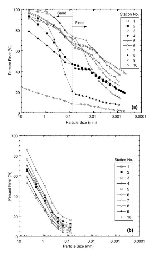
Fig. 2. Particle size distributions of the subgrade (a) and RPM (b).
