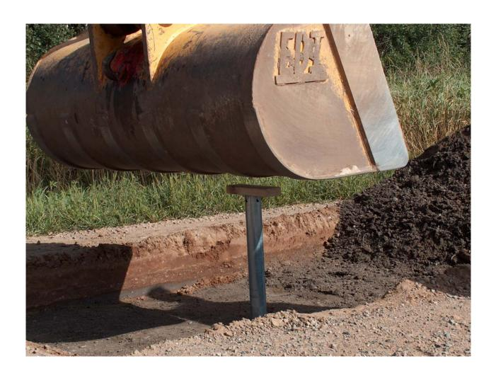
Fig A5. Collecting a sample in a thin-wall tube
