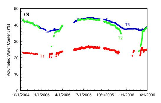
Fig. 3. Air and soil temperatures (a) and volumetric water content (b) of the SRPM and subgrade. Air temperature is shown in black. Soil temperature and water content measured at three depths: 150 mm bgs (mid-depth in SRPM) shown in red and designated as T1, 425 mm bgs (subgrade) shown in green and designated as T2, and 675 mm bgs (subgrade) shown in blue and designated as T3.
