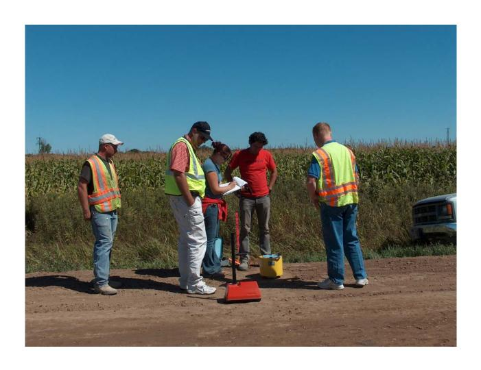
Fig A11. Nuclear gauge and SSG tests on S-RSG.
