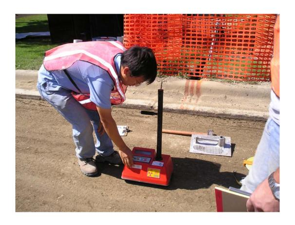
Fig. A8. Measuring water content and unit weight of SRPM after compaction.
