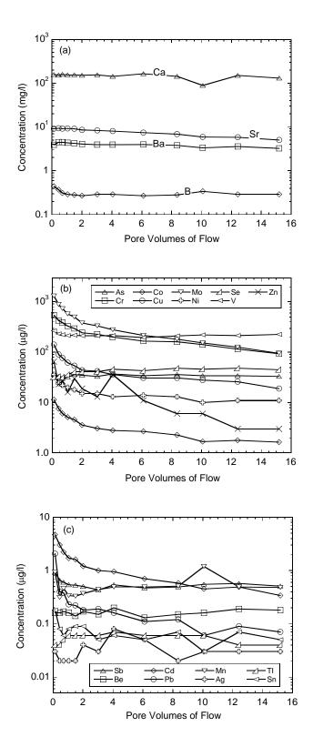
Fig. 18 Concentrations of trace elements in effluent from CLT on CH2 (Chisago Station 2): elements with peak concentrations (a) exceeding 1 mg/L, (b) elements with peak concentrations exceeding 10  $\mu$ g/L, but less than 1 mg/L, and (c) elements with peak concentrations less than 10  $\mu$ g/L.
