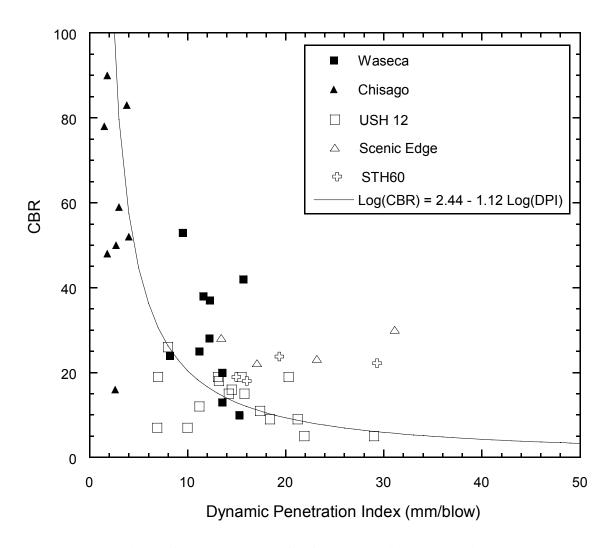
Fig. 9 CBR versus DPI for fly ash-stabilized materials
