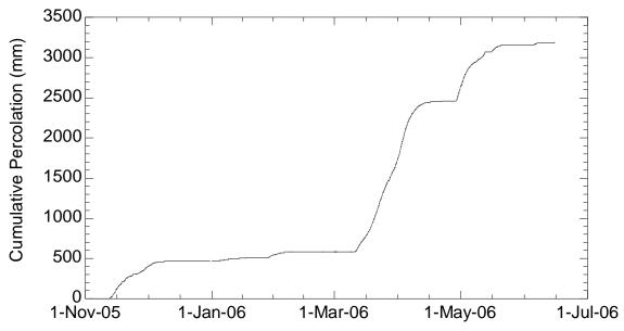
Fig. 16 Cumulative percolation into Lysimeter.
