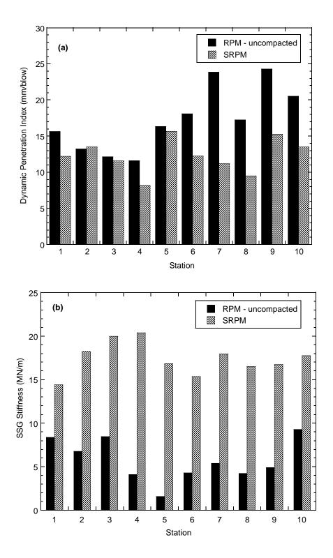
Fig. 10. Dynamic penetration index (DPI) and stiffness of uncompacted RPM and SRPM after compaction and 7 d of curing. DPI was measured with a DCP and stiffness was measured with a SSG.
