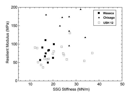
$Fig.\ 10\,Resilient\ modulus\ versus\ SSG\ stiffness\ for\ fly\ ash-stabilized\ materials$
