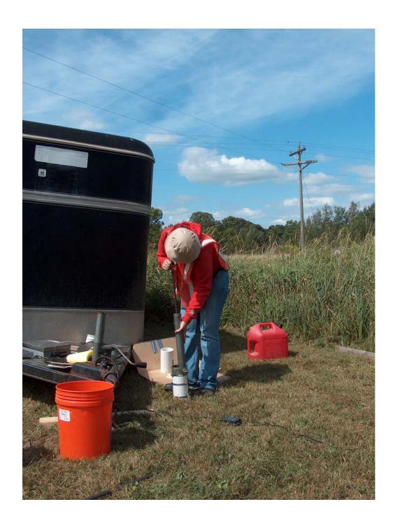
Fig A13.  $M_{\rm r}$  and CBR sample preparation of field mix soils collected with in 1-2 hour of blending process.
