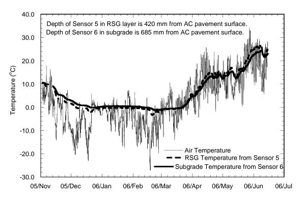
Fig. 15 Soil temperature measurements in RSG at 420 mm depth and in subgrade at 685 mm depth from the AC pavement surface.
