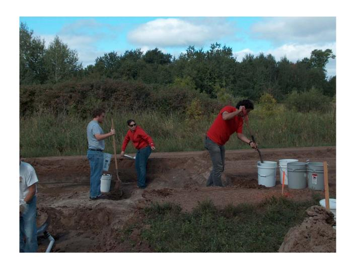
Fig A12. Collection subgrade, RSG, fly ash and S-RSG bucket samples
