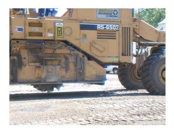
Fig. A5. Mid-section of road-reclaimer showing tines used to blend fly ash, water, and RPM.
