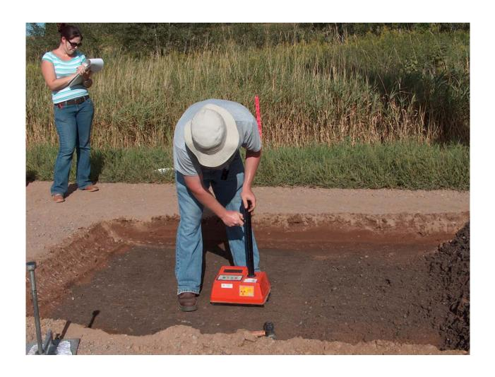
Fig A3. Measurement of water content and unit weight of subgarde.
