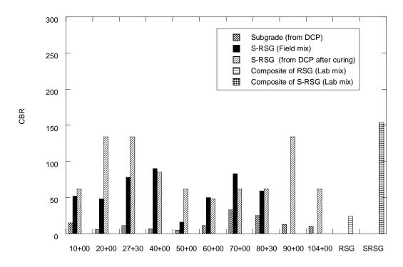
Fig. 20 California Bearing Ratio of S-RSG prepared in the field. Tests performed after 7 d of curing time.
