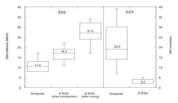
Fig. 24 Statistical evaluation of SSG and DCP test results.
