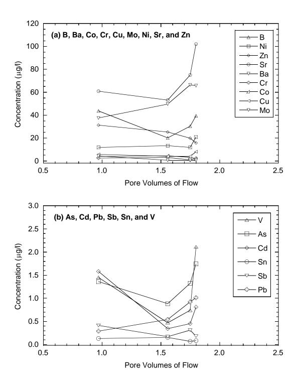
Fig. 5. Concentrations of trace elements in leachate collected in lysimeter: (a) elements with peak concentrations between 3 and 102  $\mu$ g/L and (b) elements with peak concentrations less than 2.5  $\mu$ g/L.
