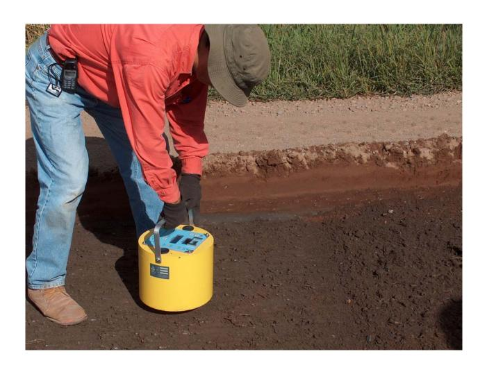
Fig A2. Soil Stiffness measurement by using SSG on subgrade.
