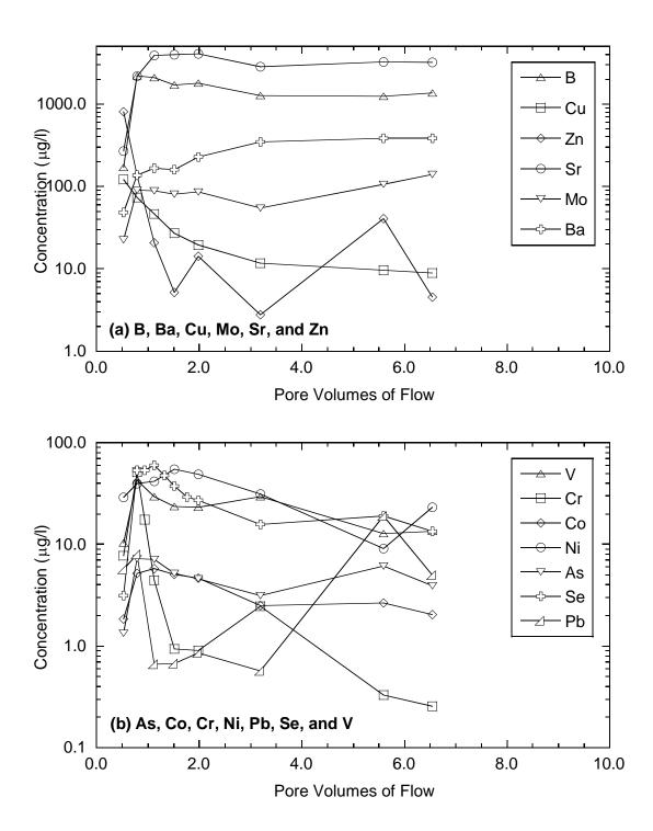
Fig. 6. Concentrations of trace elements in effluent from CLT on SRPM: (a) elements with peak concentrations exceeding 100  $\mu$ g/L and (b) elements with peak concentrations less than 100  $\mu$ g/L.
