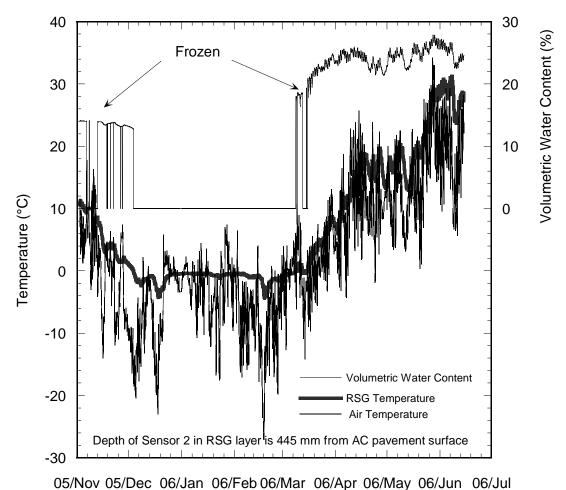
Fig. 13 Soil temperature and volumetric water content measurements in RSG at 445 mm
