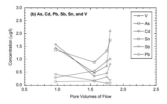
Fig. 11 Concentrations of trace elements in leachate collected in lysimeter in Waseca: (a) elements with peak concentrations between 3 and 102 g/L and (b) elements with peak concentrations less than 2.5 g/L.
