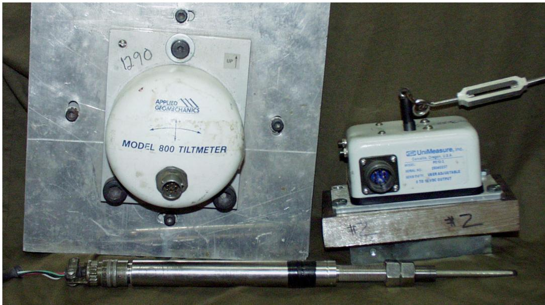
**Figure 5-3: Tiltmeter, String Potentiometer, and LVDT used for Test Displacement Measurements**
