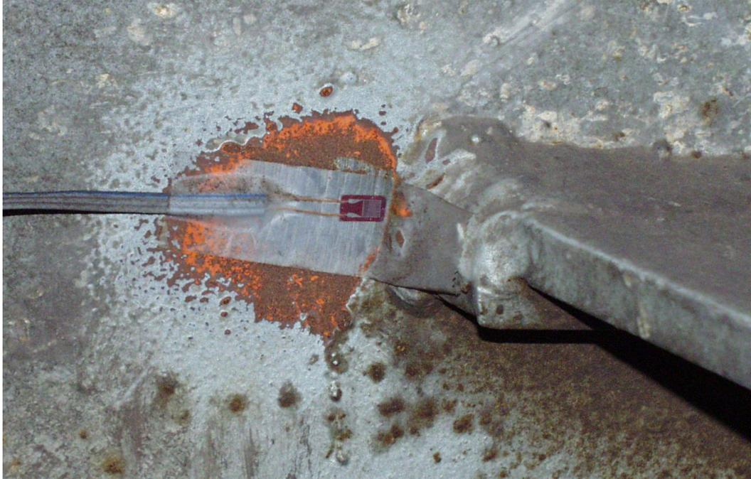
Figure 7-25: Photograph of Gusset Plate Tip Strain Gage
