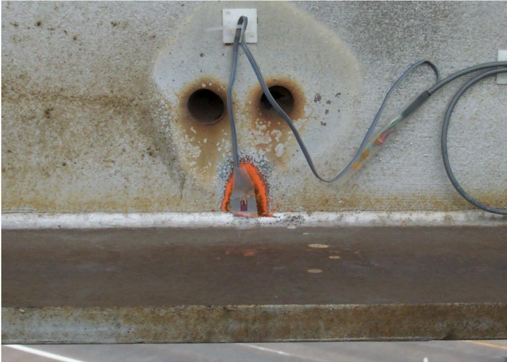
Figure 7-29: Photograph of Web Gap Strain Gage Vertically Aligned on Web
