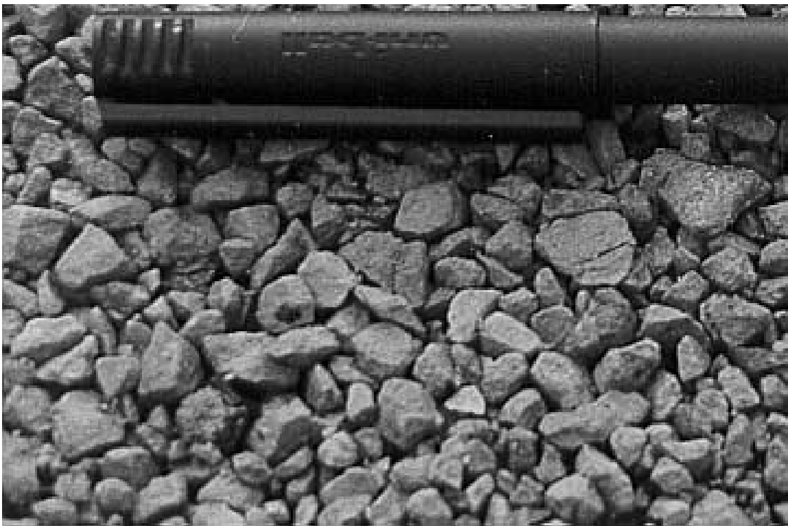
Figure 5.1. Too much aggregate (no binder is visible)
