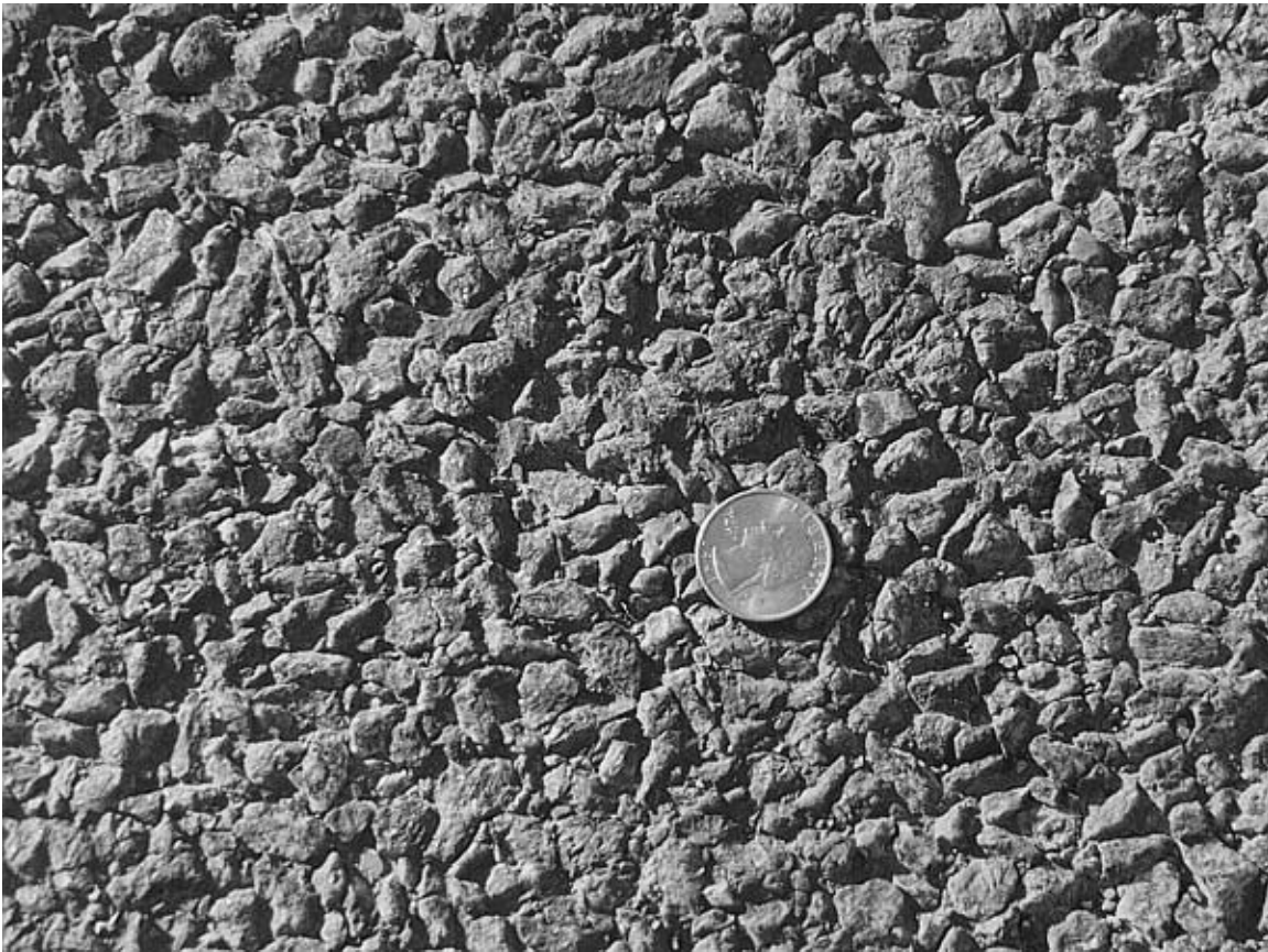
Figure 2.5. Example of a one-size FA-4 seal coat aggregate
