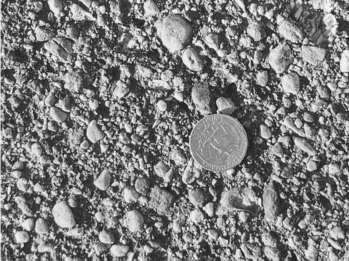
Figure 2.6. Example of a graded seal coat aggregate.
