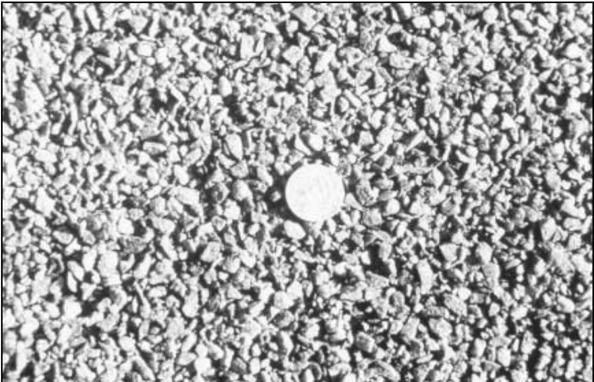
Figure 2.8. Dusty aggregate before sweeping
