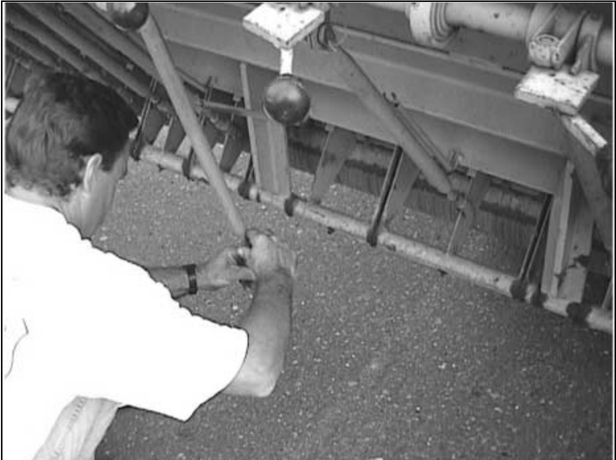
Figure 6.5. A spreader gate opening is adjusted
