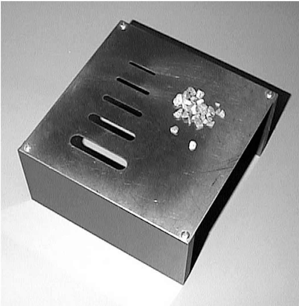
Figure 4.6. Flakiness Index Testing Plate
