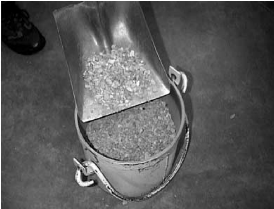
Figure 4.7. Loose Unit Weight Test
