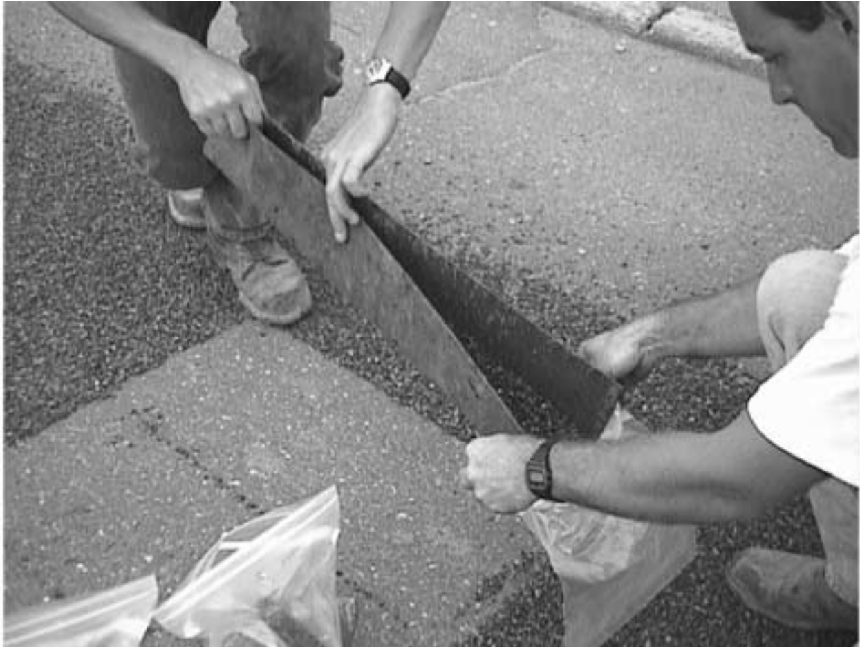
Figure 6.3. The aggregate on each mat is emptied into plastic bags
