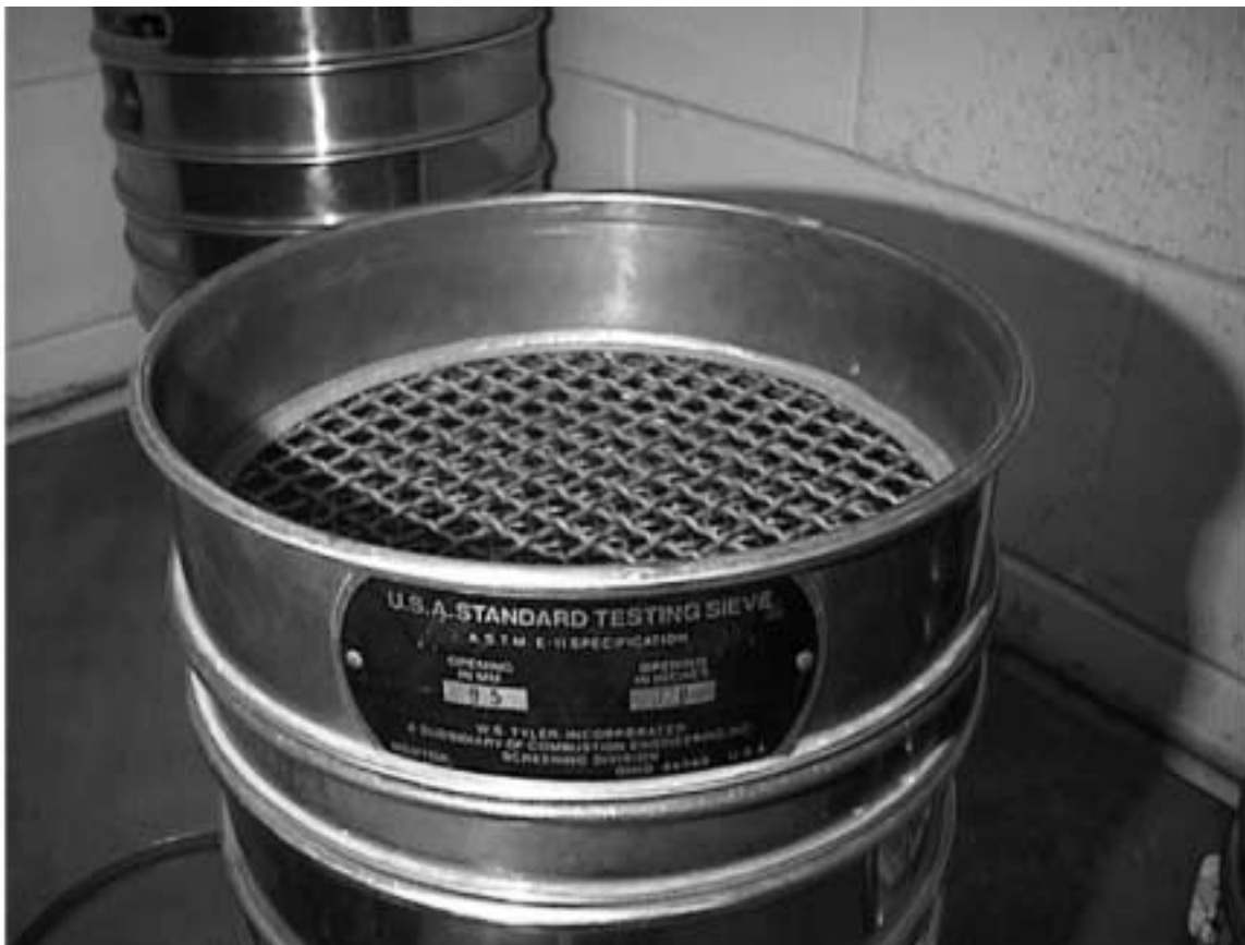
Figure 4.5. Seal Coat Sieve Nest
