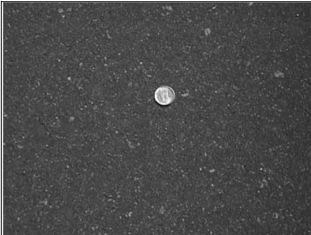
Figure 4.8. Example of a smooth, non-porous surface
