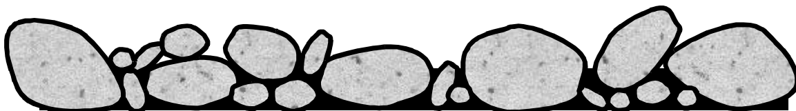
Figure 2.4. Cross section of a graded seal coat aggregate
