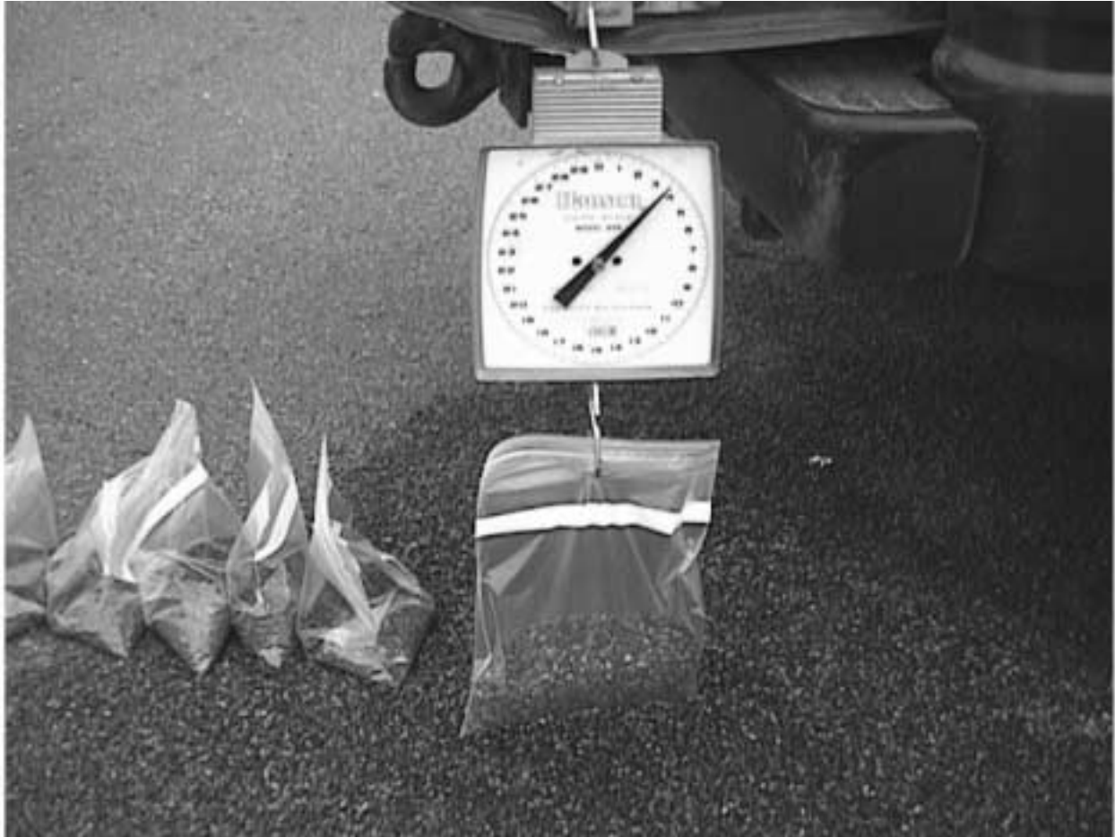
Figure 6.4. The contents of each bag are weighed and recorded
