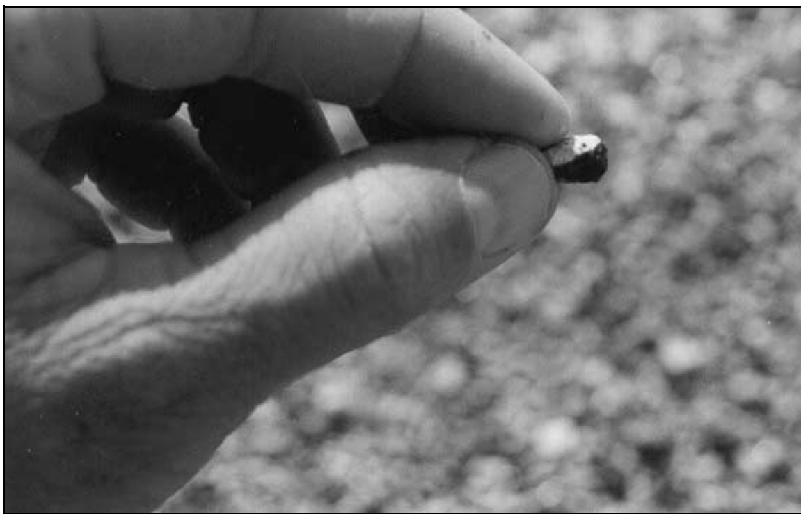
Figure 4.4. Proper embedment (~70%) into the residual asphalt.
